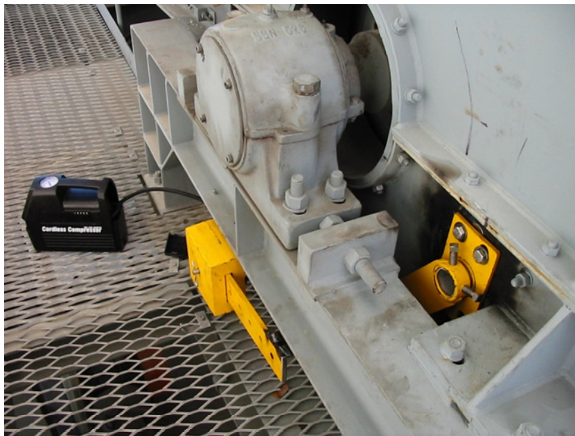
Belt cleaning system of Primary scraper mounted on self adjusting counterweight, Secondary cleaner on self adjusting counterweight, tertiary in-line air mounted system
