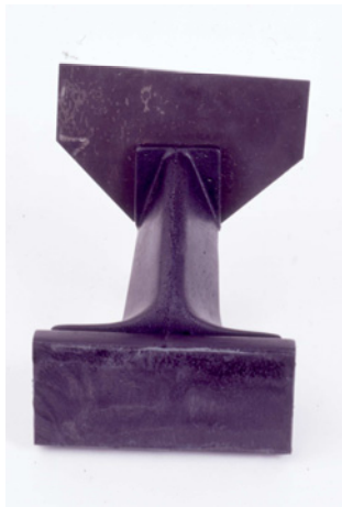
Secondary scraper blade with steel insert, suitable for counterweight self adjusting system.
