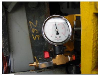
Pressure gauge to monitor pressure on inline secondary scraper on air mounted system.
