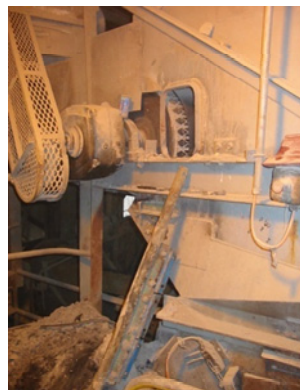
Improper Belt Cleaning System
